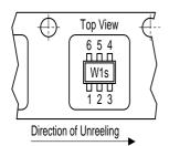
Marking on SOT-363 package (for example W1s) corresponds to pin 1 of device
