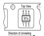
Marking on SOT-363 package (for example W1s) corresponds to pin 1 of device
