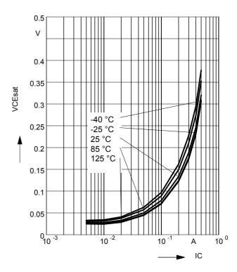
Input off voltage  $V_{i(Off)} = f(I_C)$
