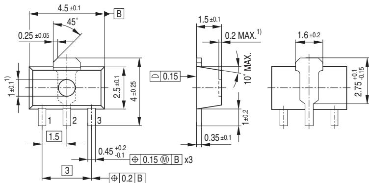
1) Ejector pin markings possible
