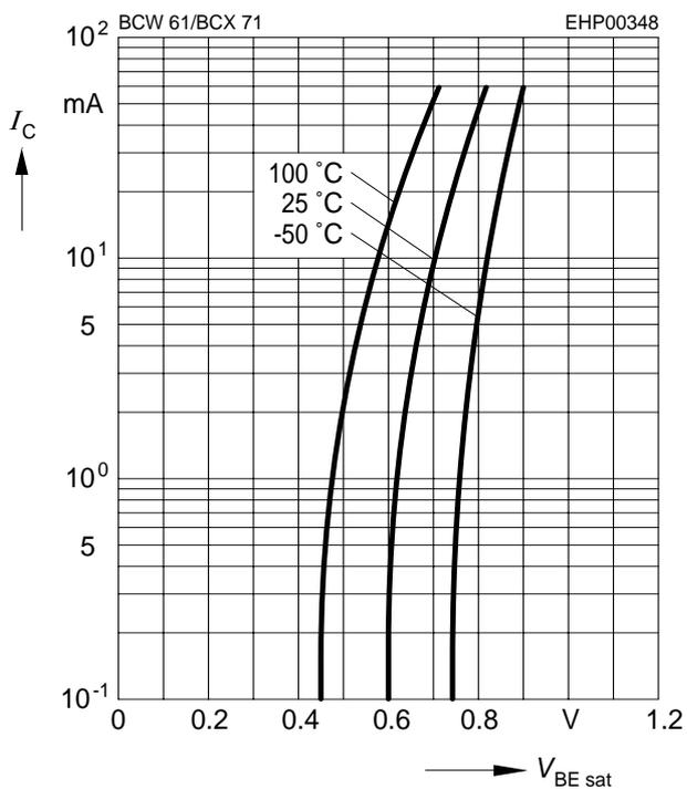
**Collector current  $I_C = f(V_{BE})$**
