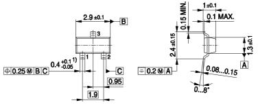
1) Lead width can be 0.6 max. in dambar area
