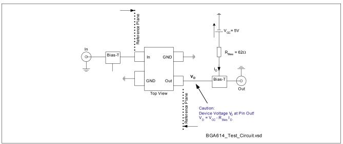
Figure 2 Test Circuit for Electrical Characteristics and S-Parameter
