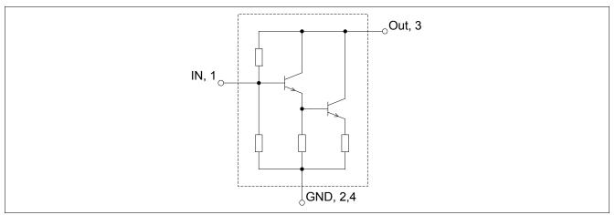
Figure 1 Pin connection
