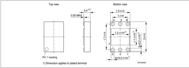
Figure 6 Package Dimensions for TSLP-7-1
