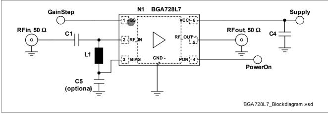
Figure 2 Application circuit of BGA728L7
