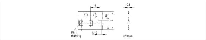
Figure 7 Tape & Reel Dimensions (Ø reel 180, pieces/reel 7500)
