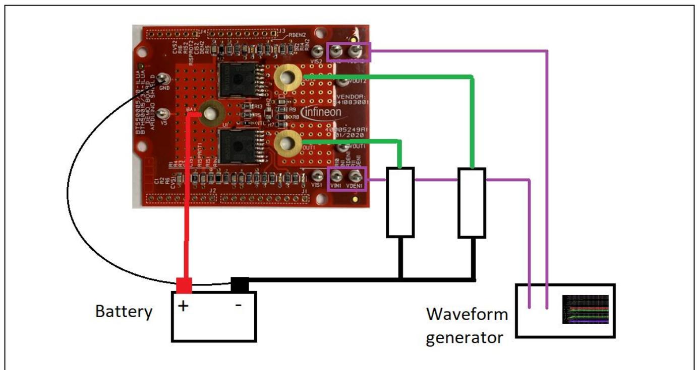
**Figure 3** Evaluation board connected to a waveform generator
