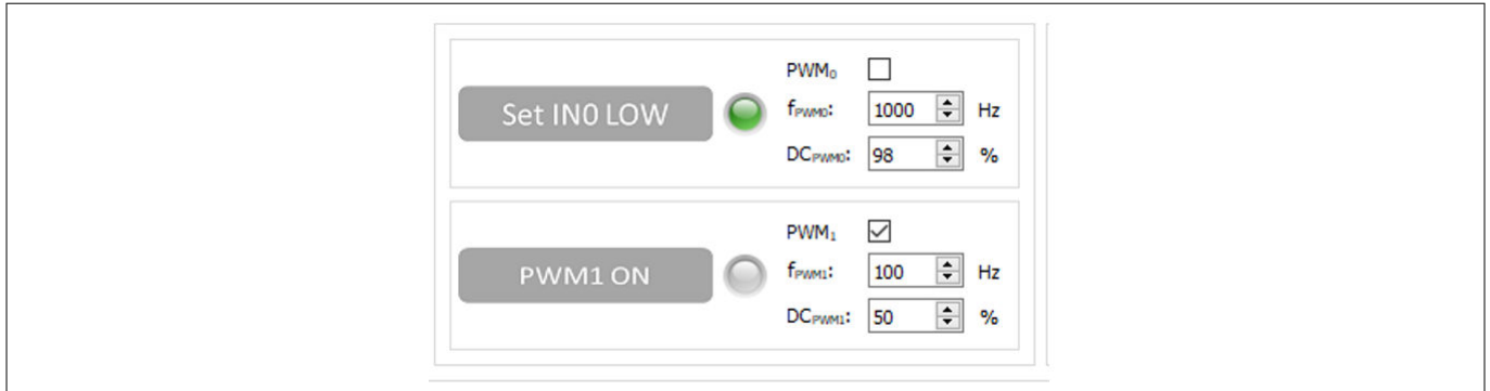
Figure 37 PROFET™ +2 12V functional view: – IN0 as logic input, IN1 as PWM input
