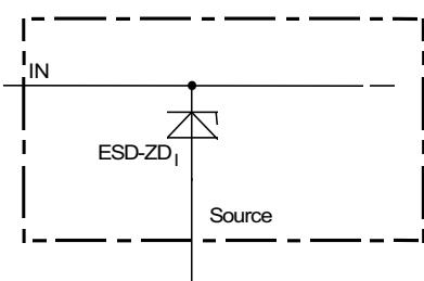
ESD zener diodes are not designed for DC current > 2 mA @  $V_{IN} > 10V$ .
