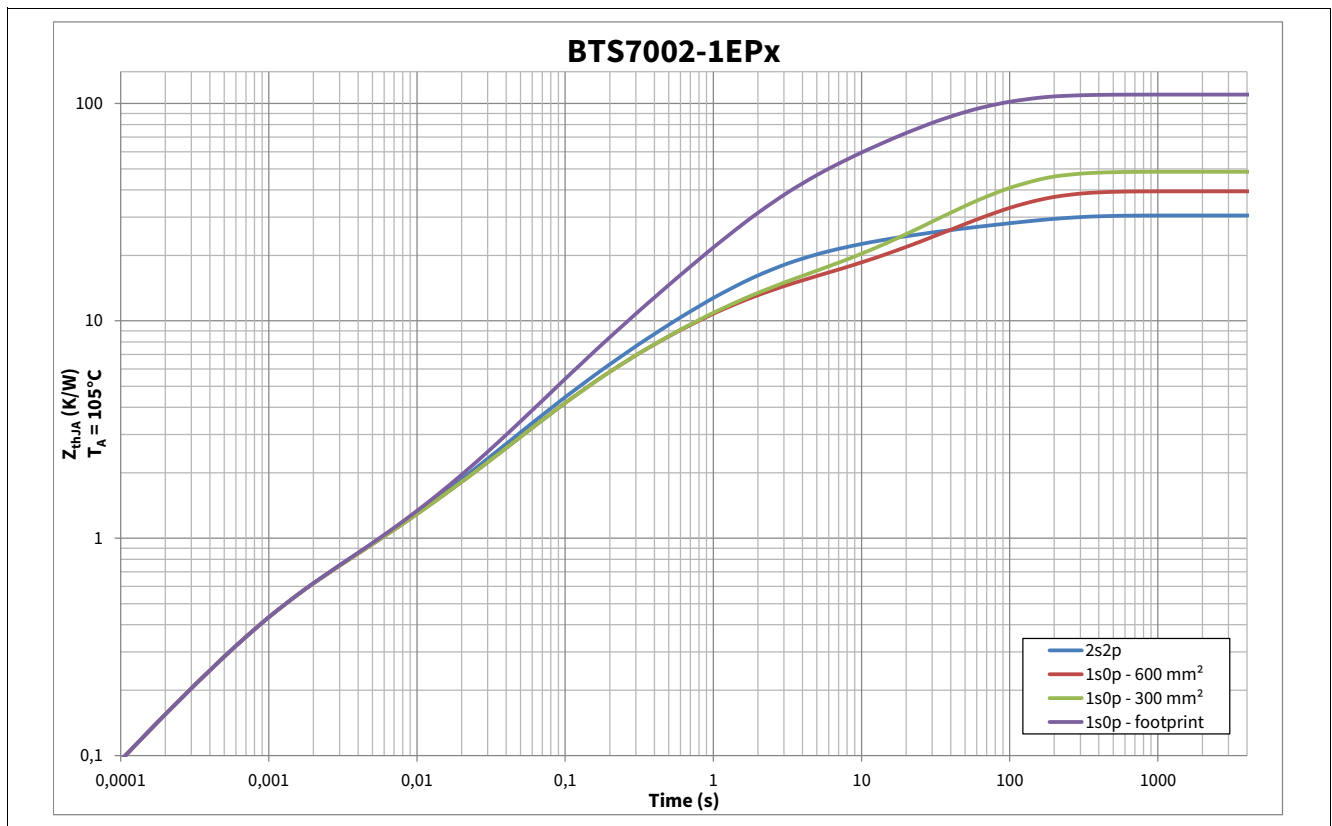
Figure 9 Typical Thermal Impedance. PCB setup according Chapter 4.4.1
