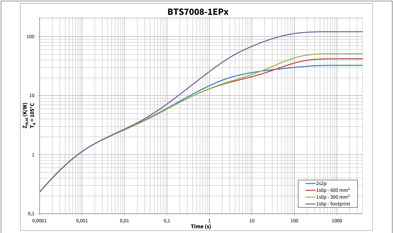
Figure 9 Typical Thermal Impedance. PCB setup according Chapter 4.4.1
