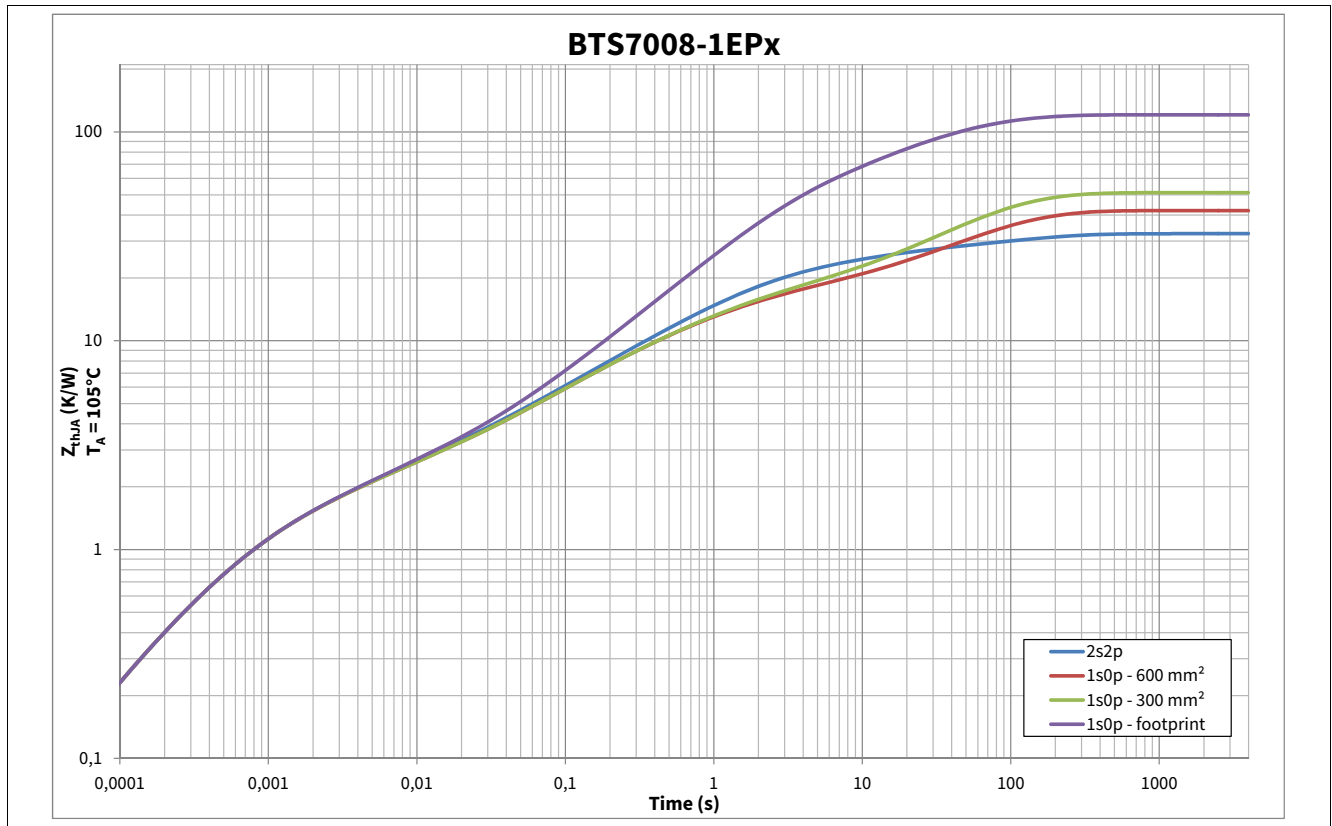
Figure 9 Typical Thermal Impedance. PCB setup according Chapter 4.4.1
