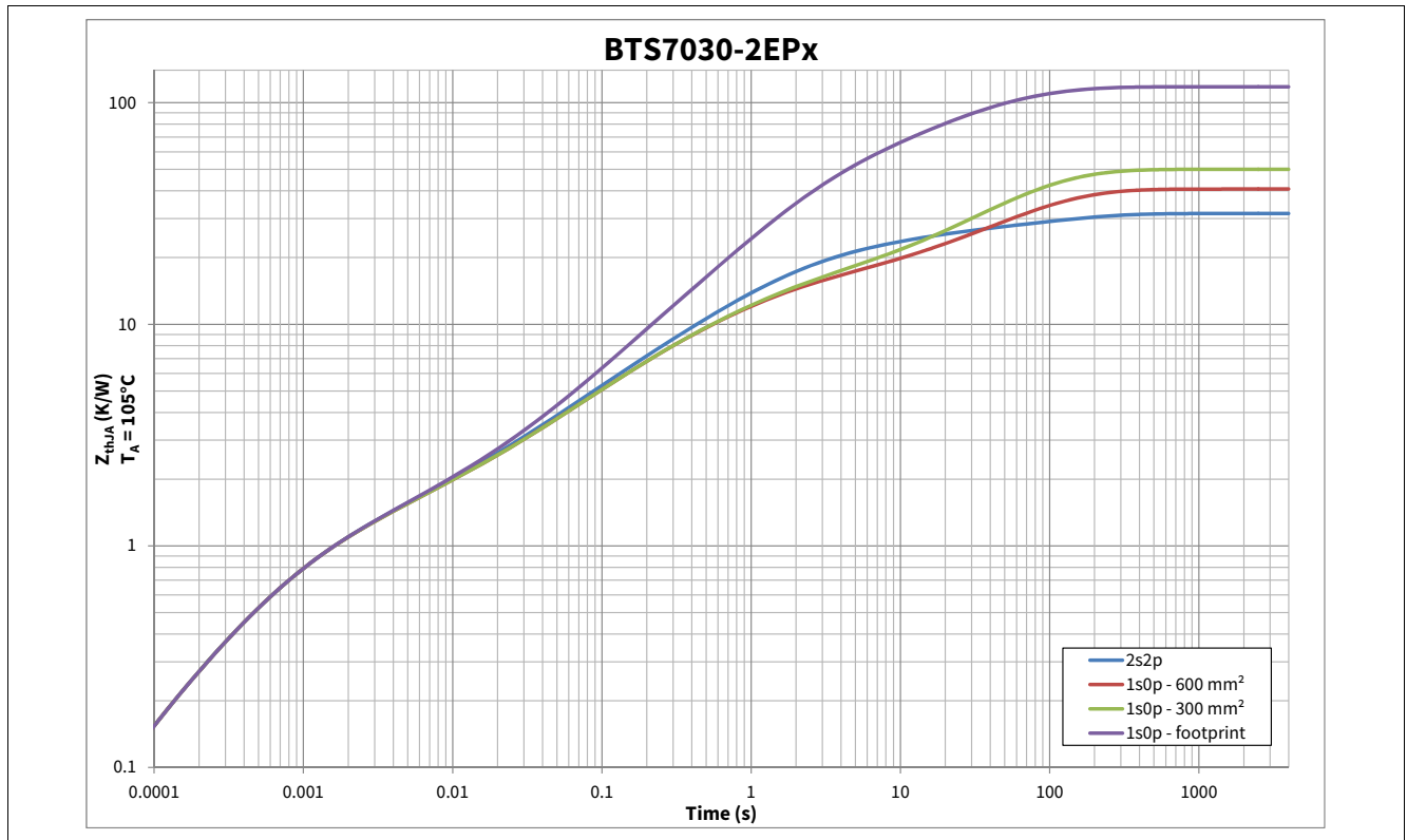
Figure 9 Typical Thermal Impedance. PCB setup according Chapter 4.4.1
