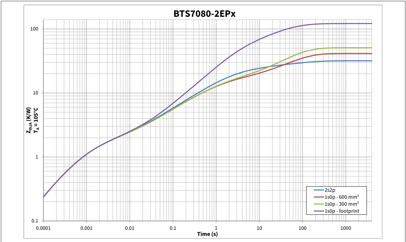
Figure 9 Typical Thermal Impedance. PCB setup according Chapter 4.4.1
