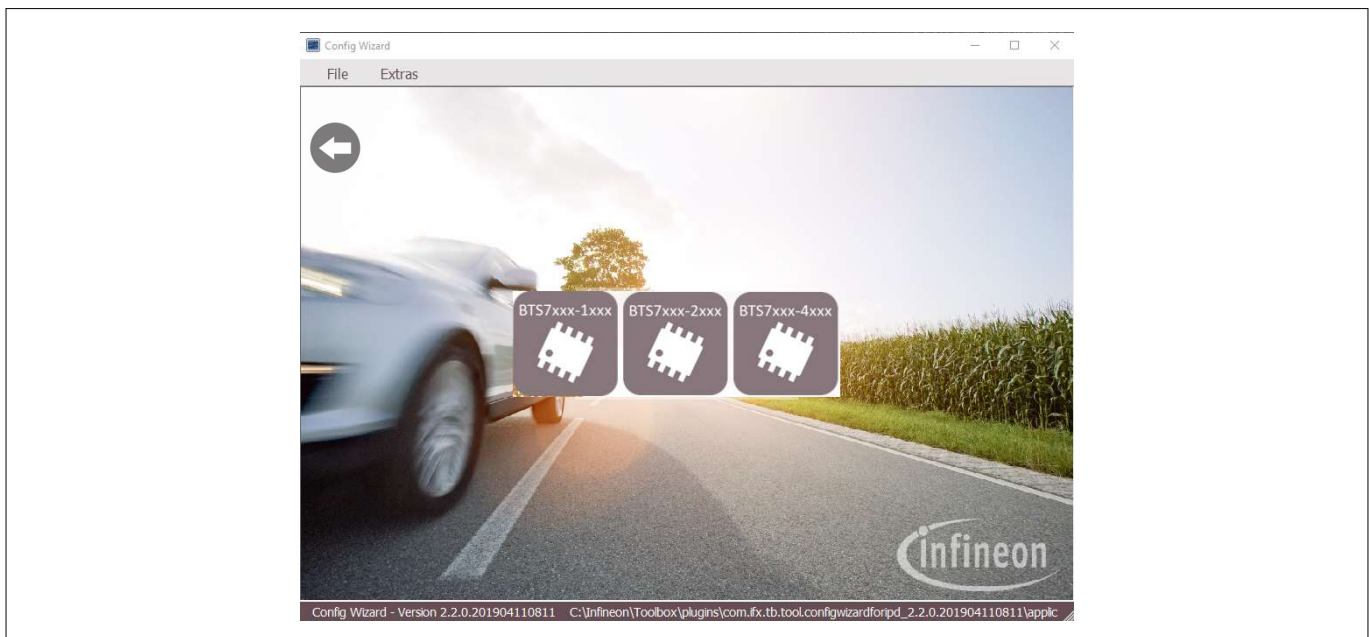
Figure 25 Config Wizard for IPD type-selection screen of PROFET™ +2 12V
