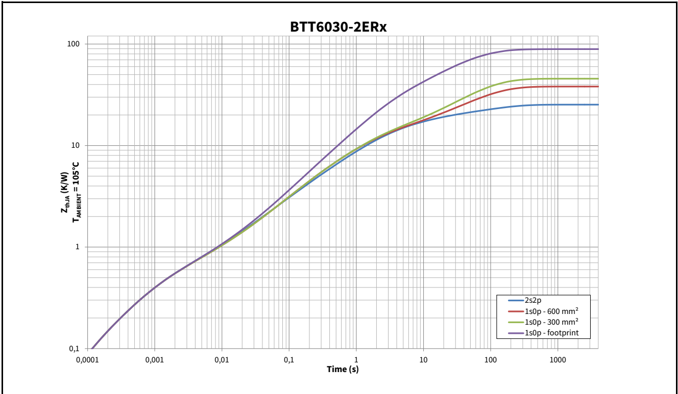
Figure 6 Typical Thermal Impedance. 2s2p set-up according Figure 4
