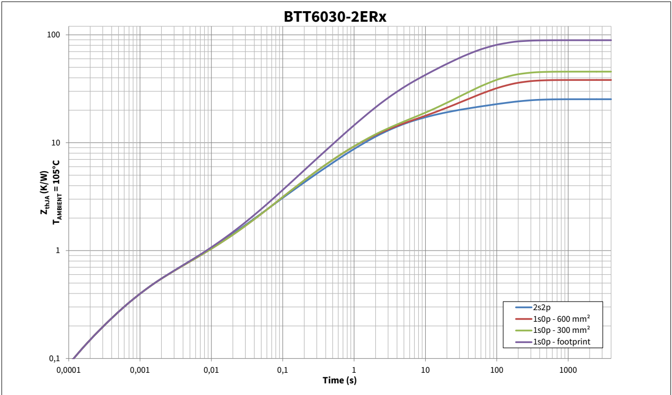
Figure 6 Typical Thermal Impedance. 2s2p set-up according Figure 4
