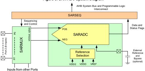
Figure 3. SAR ADC System Diagram
