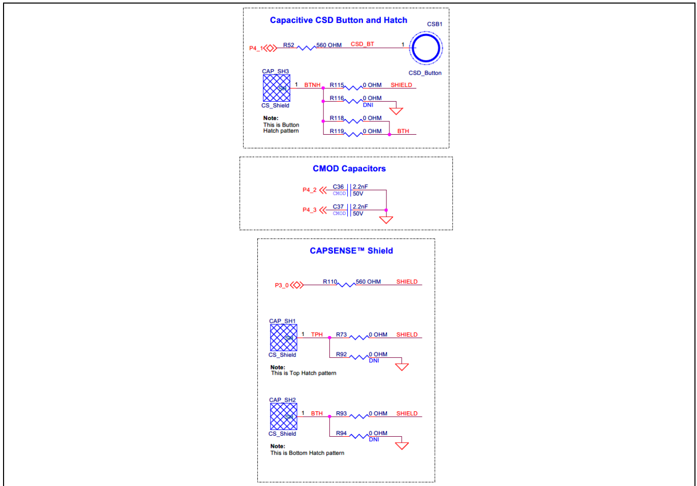
Figure 29 Schematic of capacitive sensing widgets
