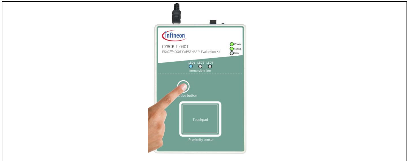
Figure 6 CAPSENSE™ button operation with LED indication
