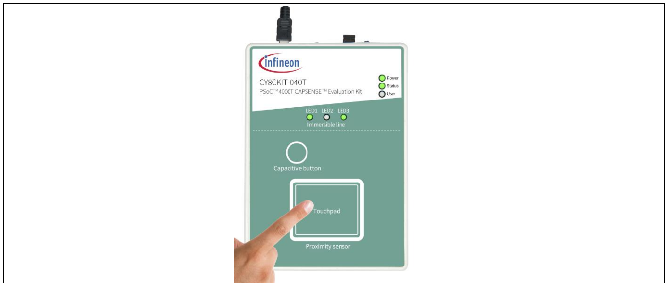
Figure 7 Capacitive touchpad operation with LED indication
