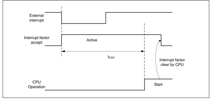
\*: External interrupt is set to detecting fall edge.
