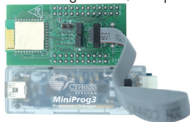
Fig 3: Programming/Debugging with MiniProg3
