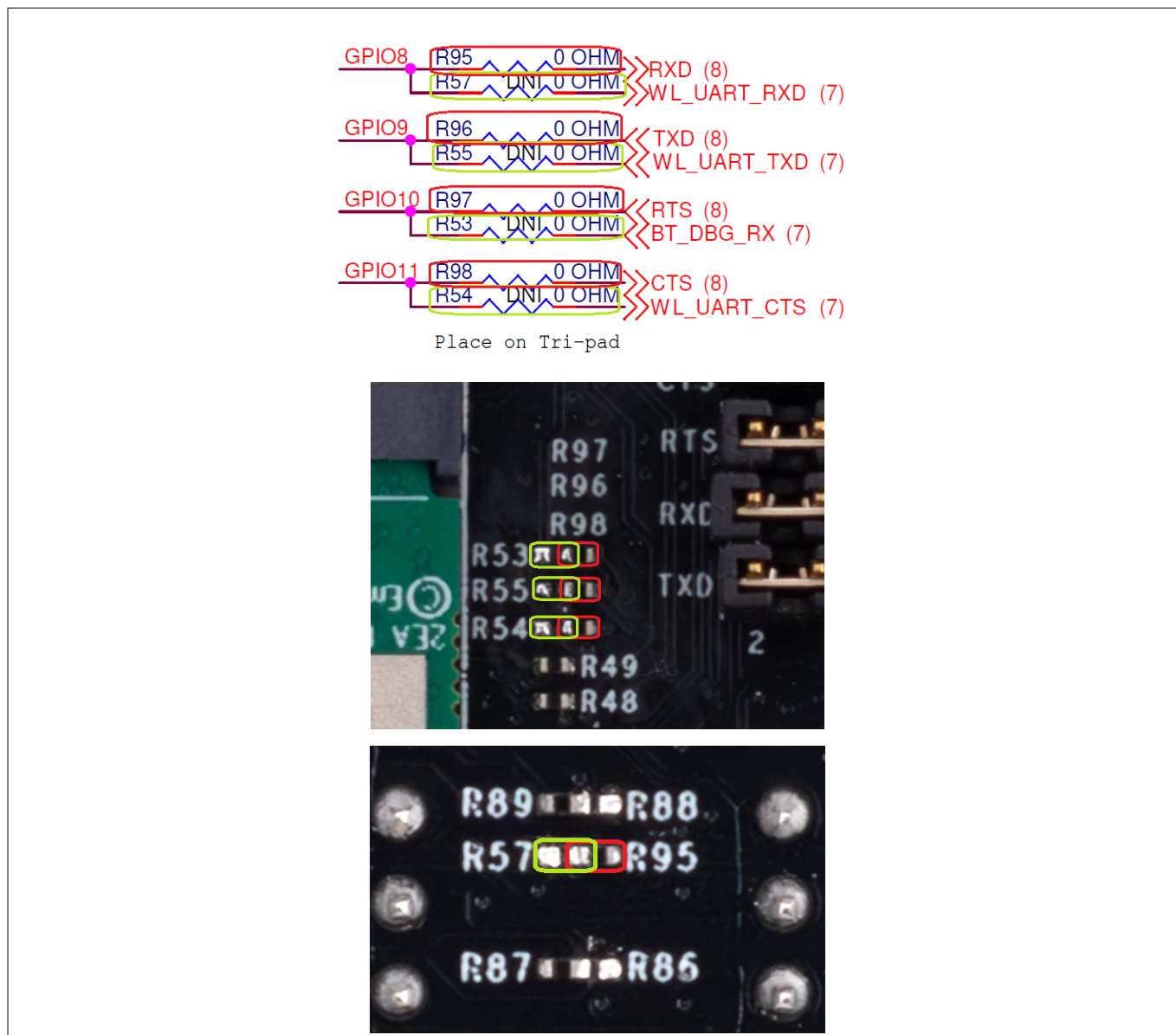
Figure 24 WL UART interface rework
