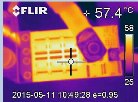
Thermal Image after 10 minutes and 250A.
