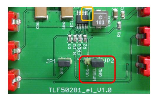
Pin 1 of JP2 is connected to OUT. Vcc is called Vbb at JP2. Please consider Vbb as Vcc, as described and listed in the datasheet.
