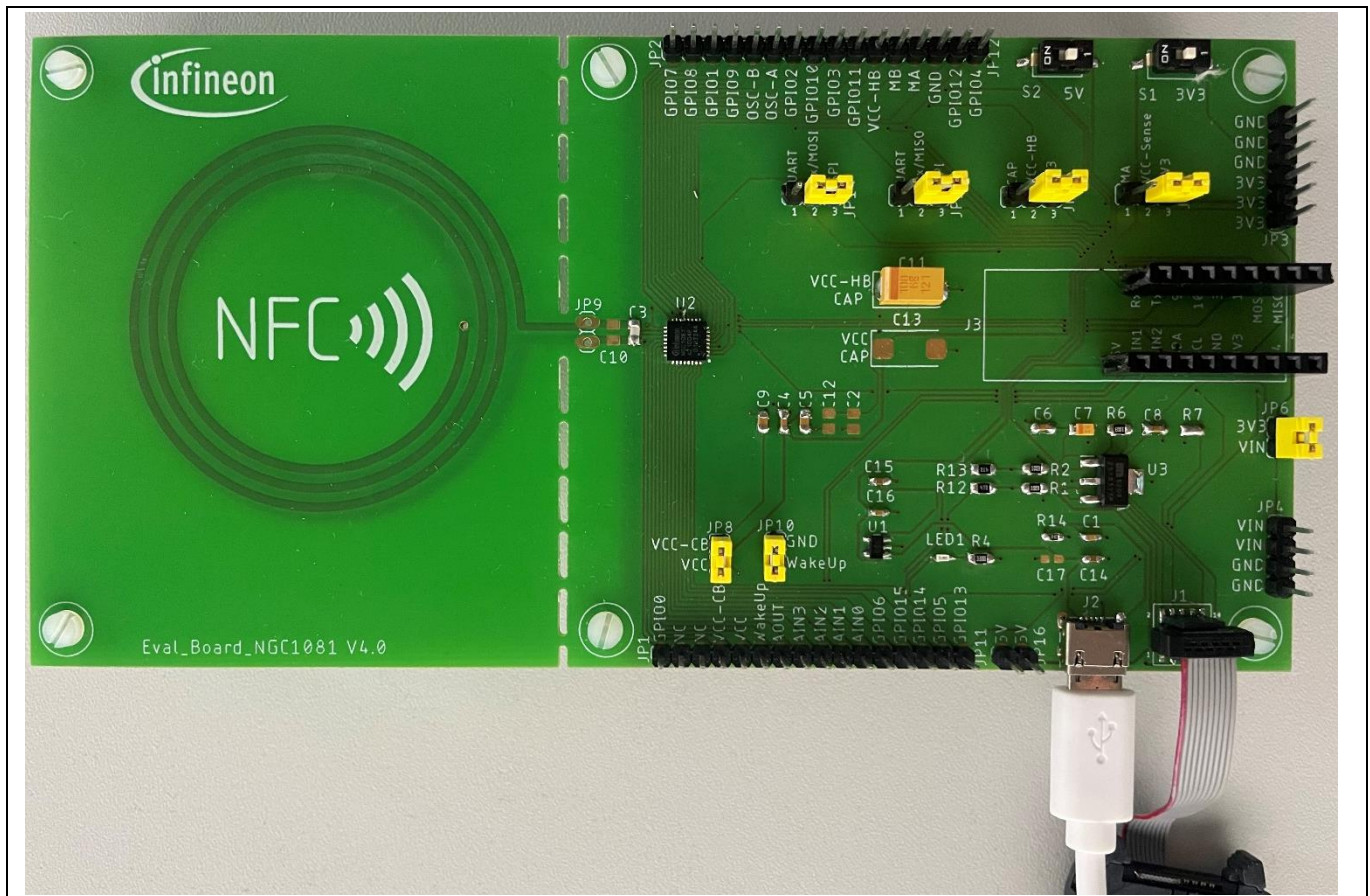
Figure 17 Connection of USB and debugger to the NGC1081
