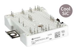
An entire PV inverter can be realized by using a single Easy 2B module. The modules incorporate an H bridge as well as a booster and a bypass diode. These modules are suitable for PV inverters with:
