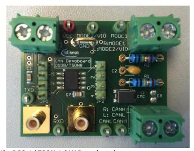
Figure 2 Photo of the DSO-8 / TSON-8 CAN Demoboard
