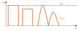
Fig. 6  $V_{WM}$  equal or higher than  $V_{signal}$
