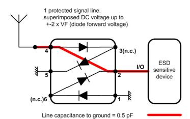
Pins 1 and 5 should be connected directly to a ground plane on the board. Pins 3, 6 are not connected. Clamped input voltage at I/O port is limited to +- 2 x VCL (clamping voltage) at positive resp. negative transients.
