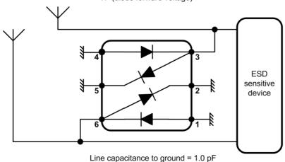
Pins 1, 2 and 4, 5 should be connected in parallel directly to a ground plane on the board. Clamped input voltage at I/O port is limited to ± VCL (clamping voltage) at positive resp. negative transients.
