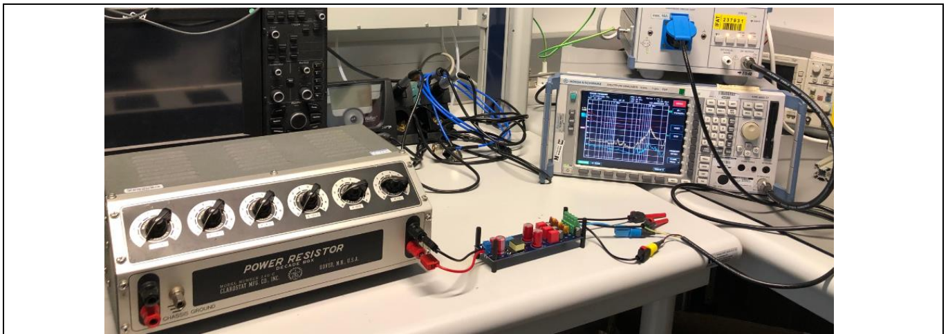
Figure 22 Conducted EMI test set-up
