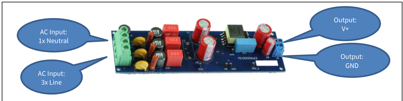
Figure 14 PCB top side showing where to connect AC input and load
