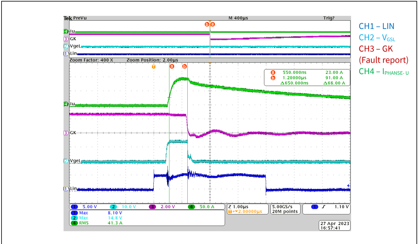
Figure 26 Short-circuit protection at V_{IN} = 600 V
