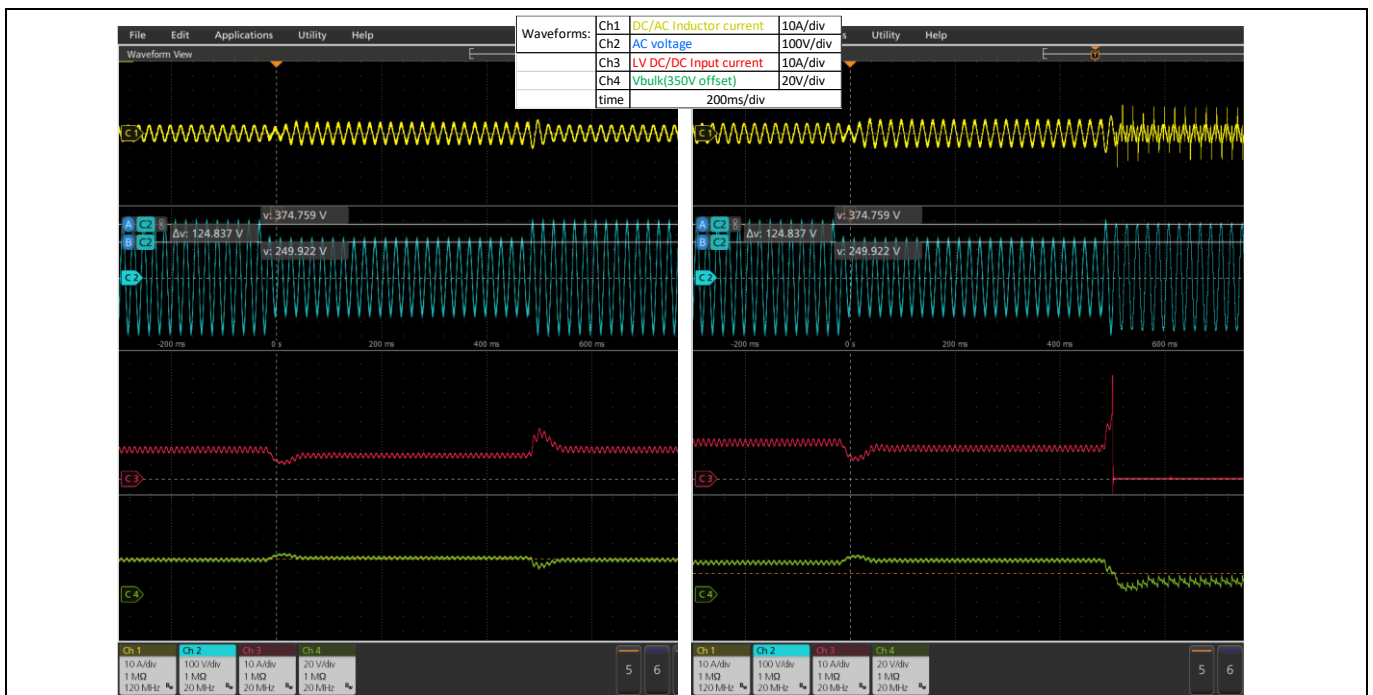
Figure 36 265 to 176 V AC voltage variation for 960 W (left) and 1200 W (right) in inverter operation
