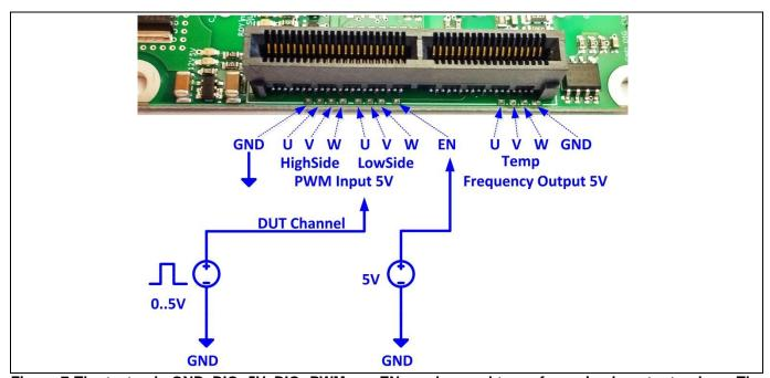
Figure 7 The testpads GND\_DIG, 5V\_DIG, PWM\_xx, EN can be used to perform simple output pulses. The testpads on the right picture simplify the access to the testpads (only revision "Sense\_V1.2" and later).
