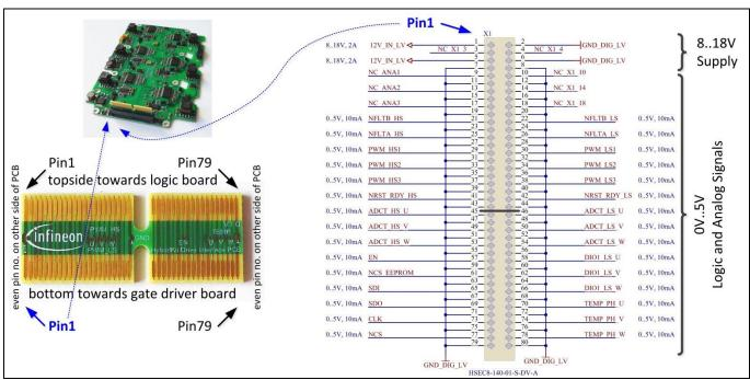
Figure 3 Board to board signal connector and pinout.
