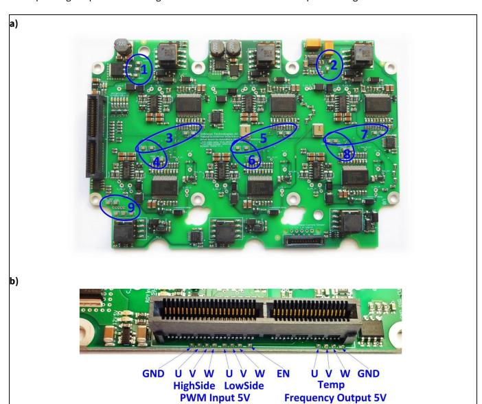
Figure 4 The testpad areas indicated on the gate driver board (a). See Table 3 for description. Important testpads are positioned also at side of the signal connector (b) (only revision "Sense\_V1.2" and later).
