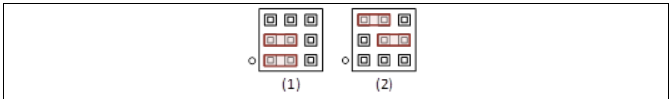
Figure 10 Double pulse test jumper settings for buck-mode (1) and boost-mode (2)
