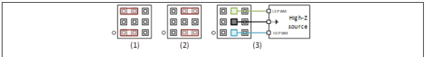
Figure 3 Jumper J1 settings for dual 50 \Omega logic inputs (1), single high-side 5V logic input (2), and dual 5 V High-Z terminated logic inputs (3)
