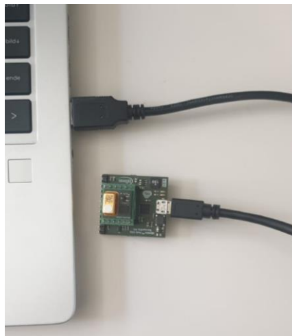
Figure 7 XENSIV™ PAS CO2 Sensor2Go Evaluation kit connection to PC via micro USB cable
