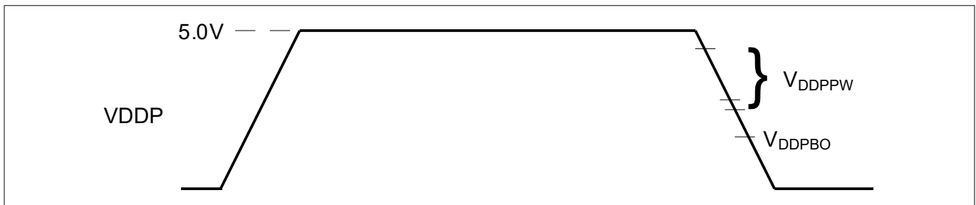
Figure 11 Supply Threshold Parameters
