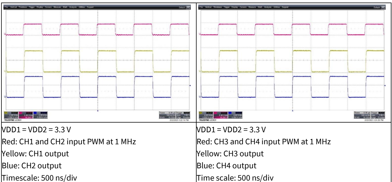
Figure 9 Typical input and output waveforms of EVAL_ISO_4DIR1400H
