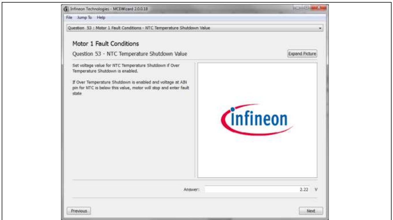
Figure 18 External temperature sense input configuration in MCEWizard
