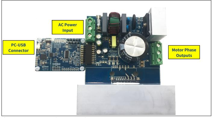
Figure 4 System connection example using EVAL-M1-CTF610N3 and EVAL-M1-101T
