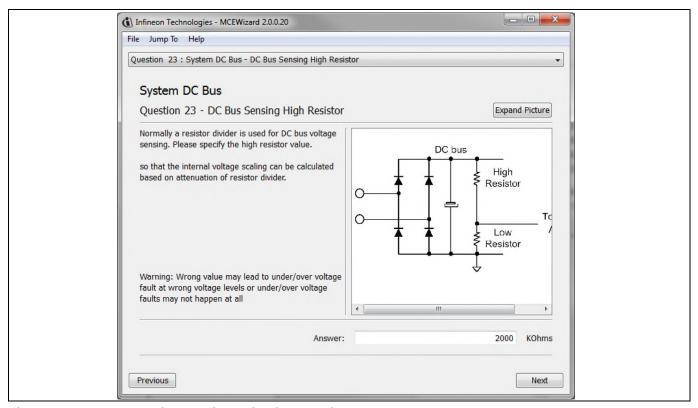
Figure 12 DC bus sensing configuration in MCEWizard
