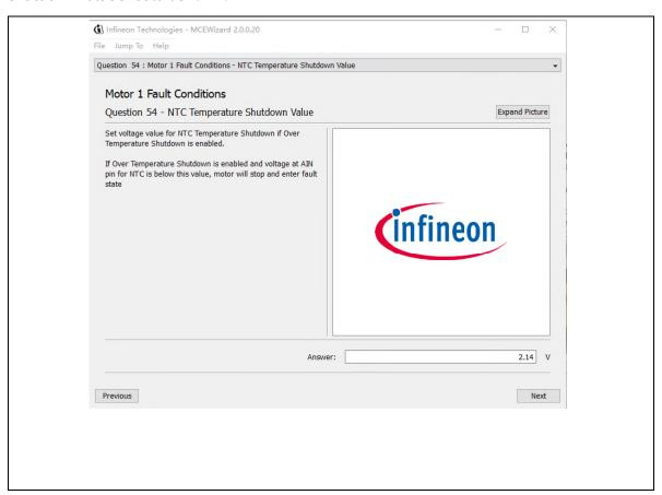
Figure 20 External temperature sense input configuration in MCEWizard
