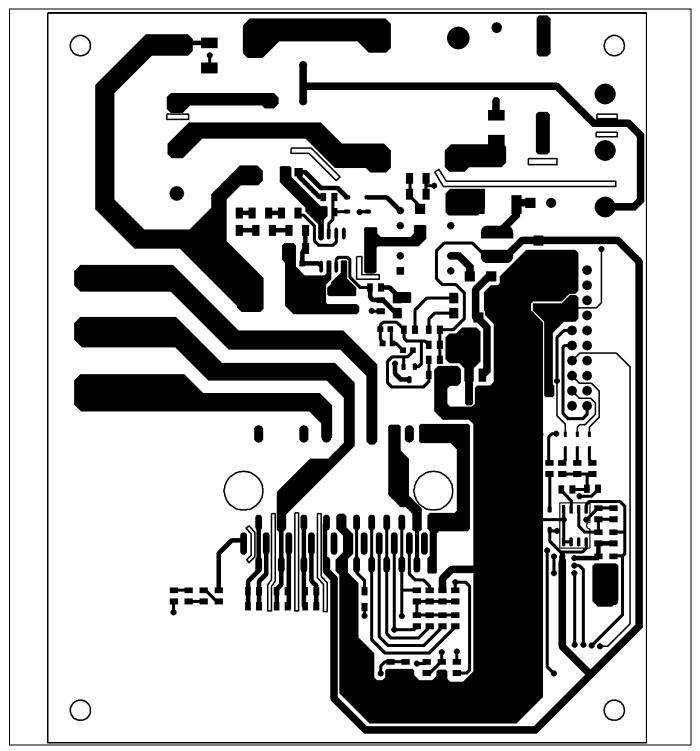
Figure 28 Bottom layer routing of the EVAL-M1-CTF610N3
