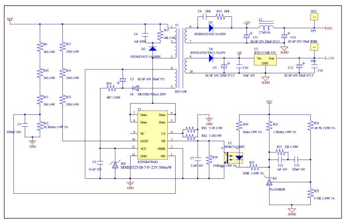
Figure 24 Auxiliary Power Supply Section Schematics for EVAL-M1-CTF610N3
