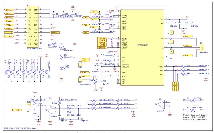
Figure 23 Inverter Section Schematics for EVAL-M1-CTF610N3
