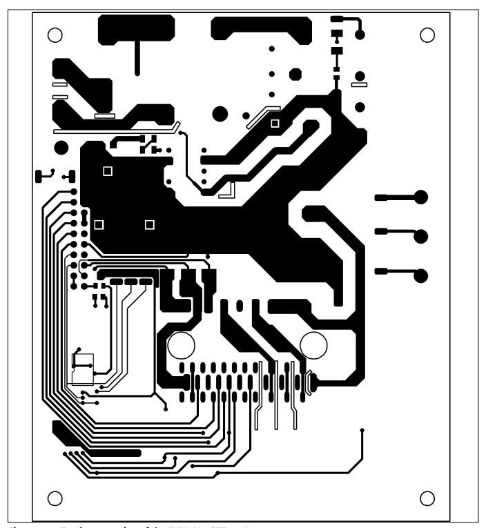
Figure 27 Top layer routing of the EVAL-M1-CTF610N3
