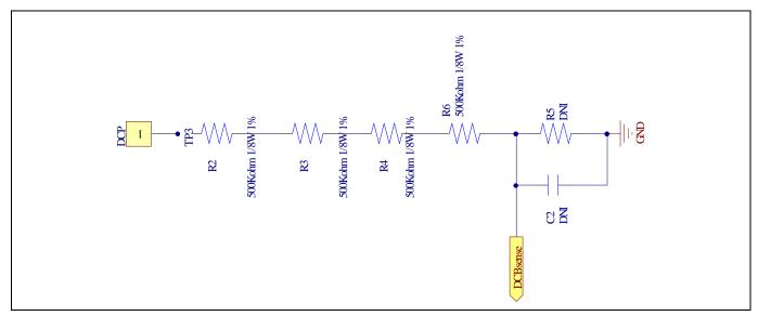
Figure 11 DC bus sense resistor on EVAL-M1-CTF610N3 evaluation board
