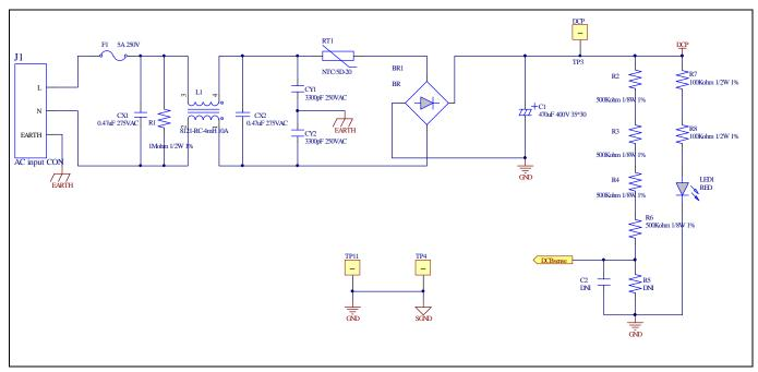
Figure 22 AC Linear Section Schematics for EVAL-M1-CTF610N3
