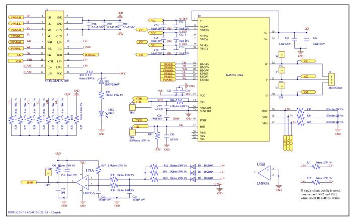
Schematic of the 3-phase inverter section using CIPOS™ Tiny IPM on EVAL-M1-CTF610N3
