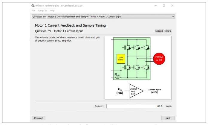
Figure 15 Current feedback configuration in MCEWizard for EVAL-M1-101T and EVAL-M1-CTF610N3
