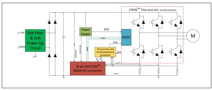
Figure 1 The Block Diagram of the EVAL-M1-CTF610N3
