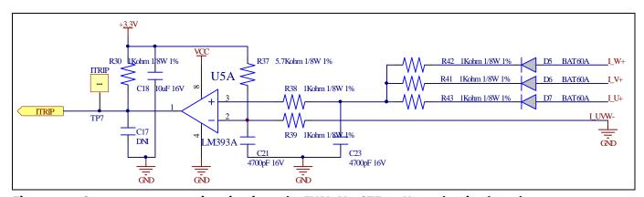
Figure 16 Overcurrent protection circuit on the EVAL-M1-CTF610N3 evaluation board
