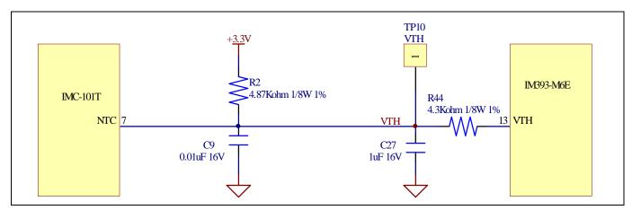
Figure 19 Overtemperature protection circuit schematic for EVAL-M1-CTF610N3 and EVAL-M1-101T
