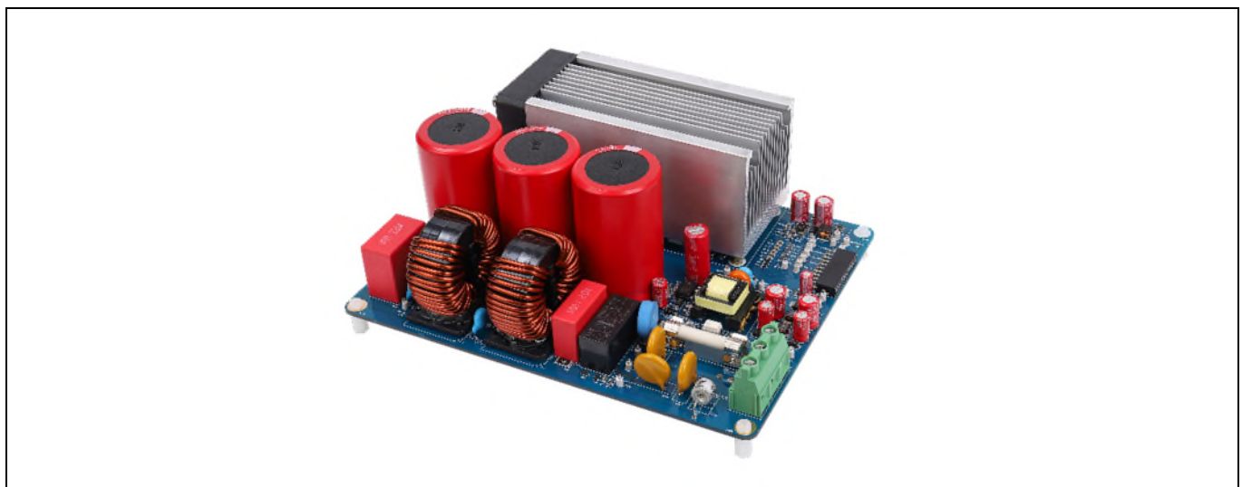
Figure 1 The iMotion™ MADK evaluation board for IM323-L6Gx CIPOS™ Tiny IPM
