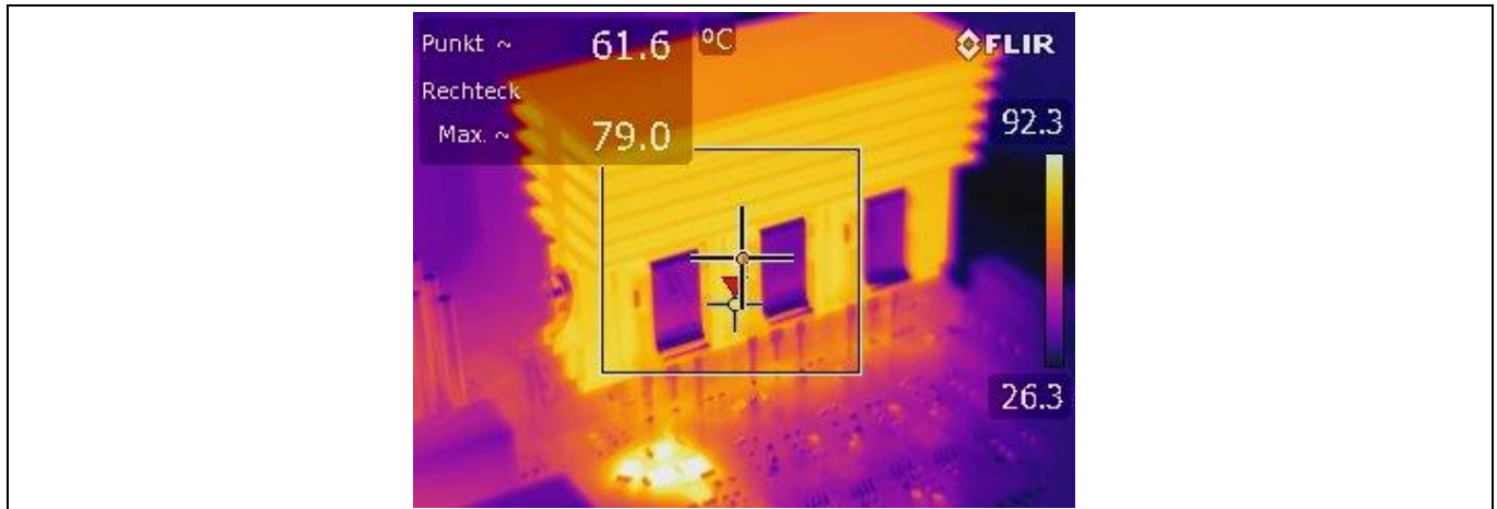
Figure 30 Thermal image the left power MOSFETs
