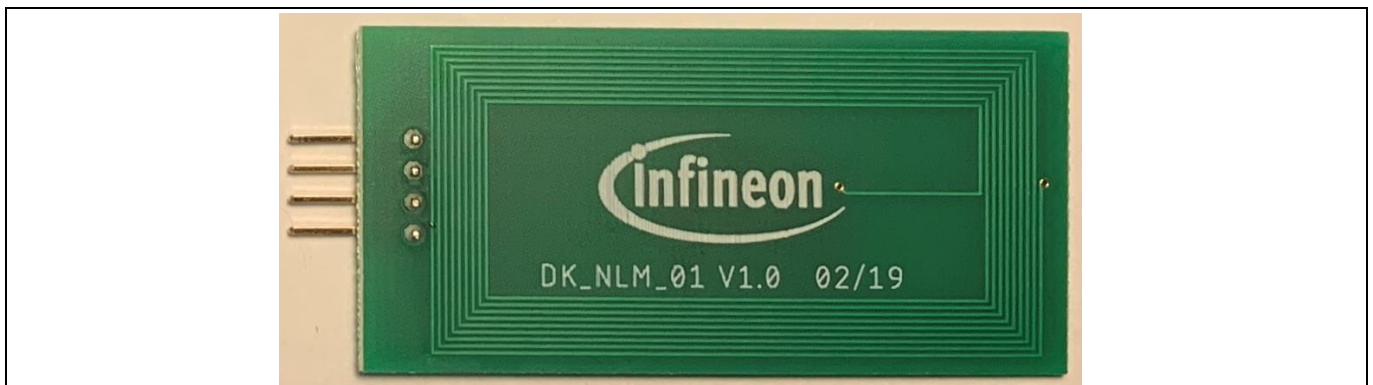
Figure 27 Top view of DK_NLM_01 with NFC antenna
