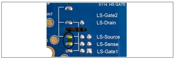
Figure 7 Bottom view power connector
