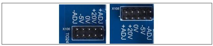
Figure 6 Drive voltage jumpers
