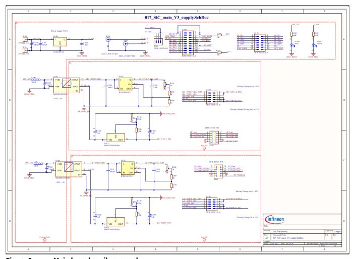
Figure 9 Main board auxilary supply
