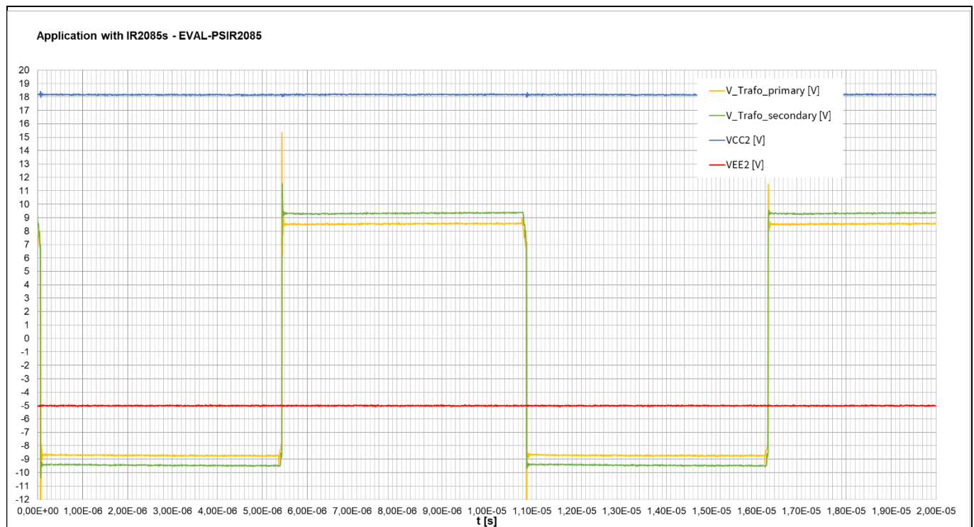
Figure 11 Normal operation of the power supply board
