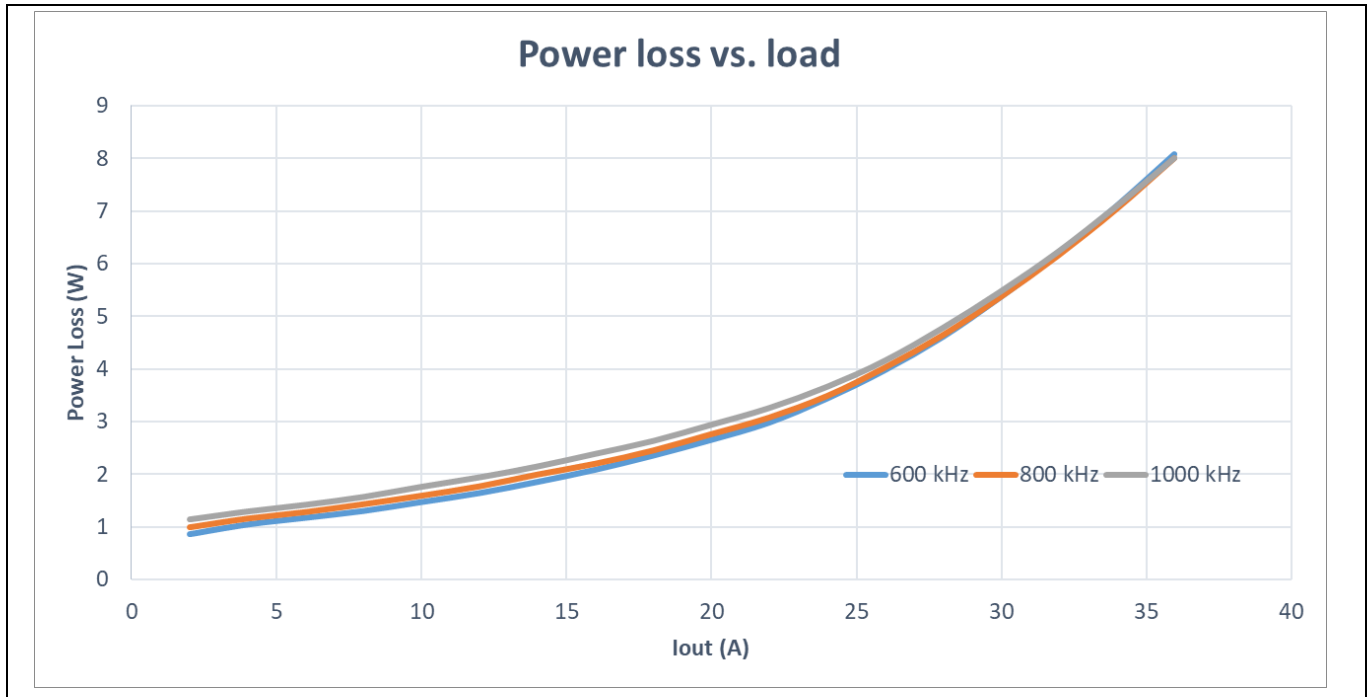
Figure 31 Power loss vs. load current without airflow in FCCM with external V CC (12 V P VIN , 3.3 V V OUT , no airflow, 150 nH, 600 kHz/800 kHz/1000 kHz, T a = 25°C)
