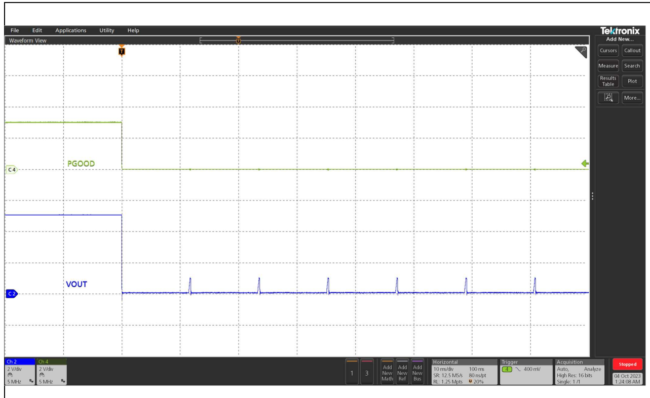
Figure 15 Short circuit and UVP (Hiccup), (Ch2: Vo, Ch3:PGood)
