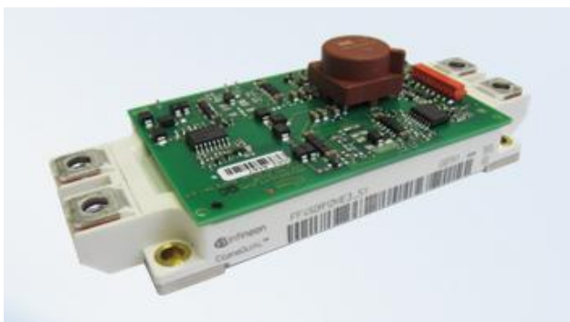
Figure 1 The 2ED100E12-F2 Evaluation Driver Board mounted on the top of the EconoDUAL™ 3 module
