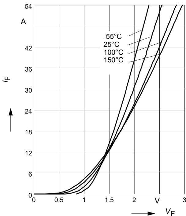
**4 Typ. diode forward voltage**
